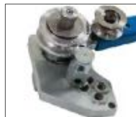
UNIFLEX insert – marking tool (ferrule position marking increases productivity and improves safety in hose sizes up to 2".
