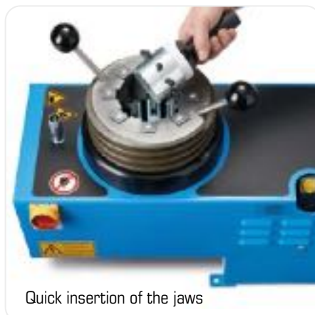
SH 7 with closed dies and QDC
