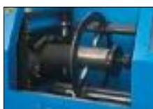
Double skiving tool with hose.
