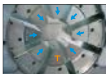
The fixed 6- o'clock die makes safe and low-force positioning of the workpiece possible.
