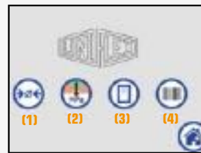
More parameters to comfortably conduct serial pressing. Selection menu for pressing sorted by press dimension/pressure, using production data from the database or by scanning with the barcode scanner.
