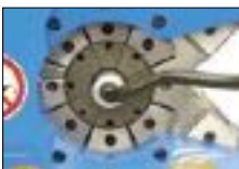
Radial insertion of workpieces, catering even to 90° bends.
